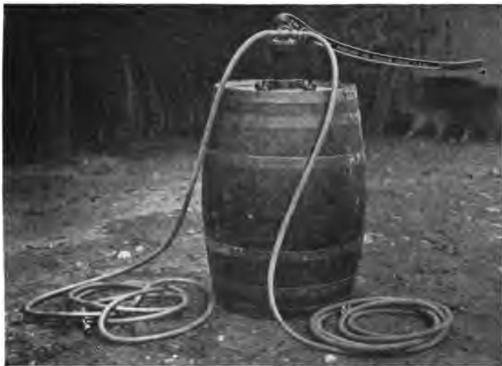
FIG. 148.—An inexpensive spray pump with two leads of spray hose. More useful in the home orchard than in the garden. (New Jersey Station.)
